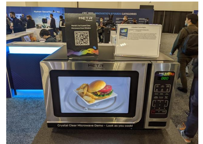
NANOWEB® EMI Shielding (right) provides clear visibility while protecting against harmful radiation.
